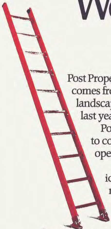
In trenches, escape ladders placed every 25 feet help workers get out more quickly.
