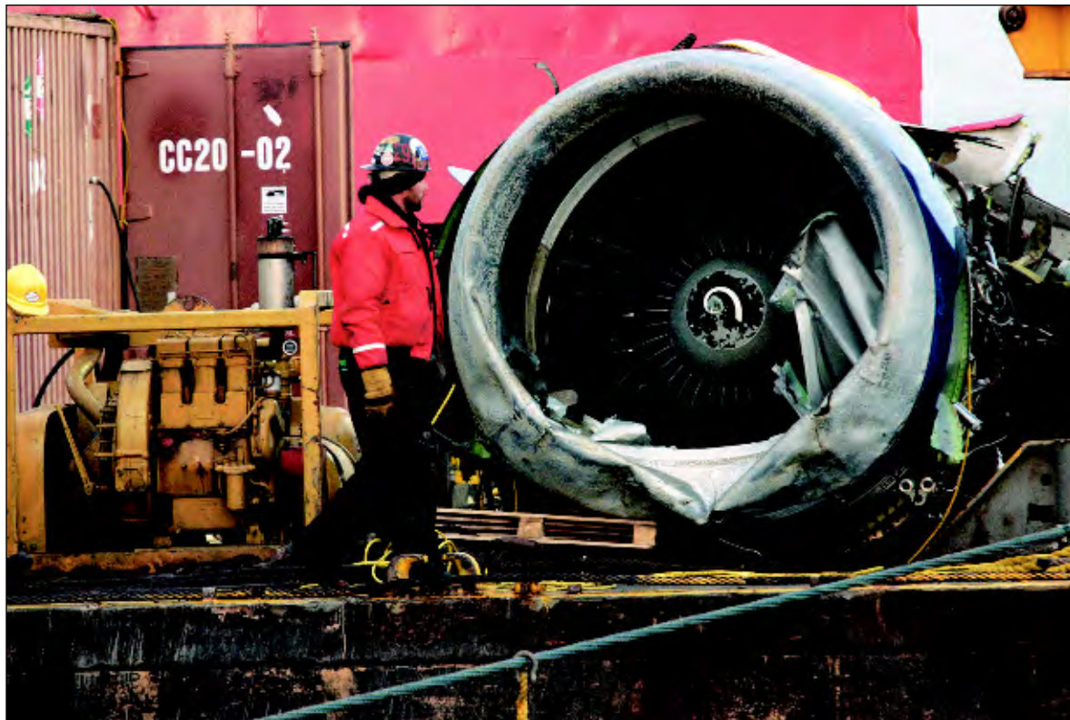
The engine of US Airlines Flight 1549 rests on a barge on the Hudson River after the plane was forced to make an emergency landing after it collided with a flock of birds in January 2009.
