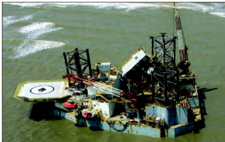
An oil platform in the Gulf of Mexico was ripped from its mooring in August 2005 after Hurricane Katrina passed through the area.
