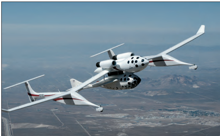
SpaceShipOne is lifted over California's Mojave Desert by a launch aircraft in advance of its historic flight on June 21.
