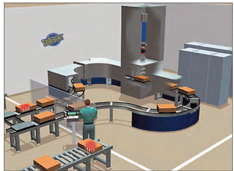
The U.S. Postal Service is buying up to 20 SureBeam systems from Titan Corp. The system uses linear accelerators to sterilize parcels.
