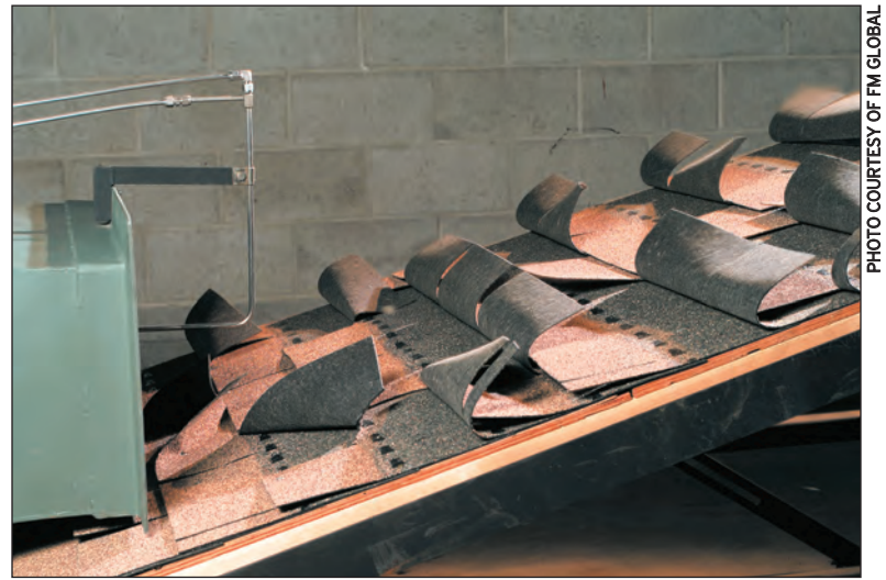
FM Global uses a wind machine at its research campus that can simulate a category 5 hurricane, generating wind speeds up to 160 mph, to test building designs and materials.
