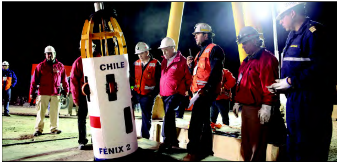
The 33 trapped Chilean miners escaped the mine last week in a single-man rescue pod through a shaft only around 28 inches in diameter.
