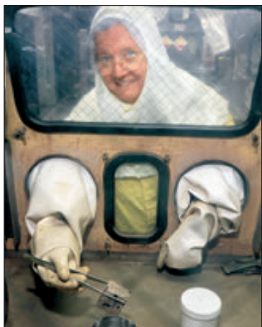
Extensive equipment, such as this glovebox, shields scientist Susan Jones from radiological exposure in handling plutonium.
